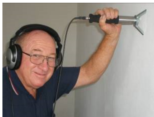
Fig.6 listening to a leaking pipe through the wall
