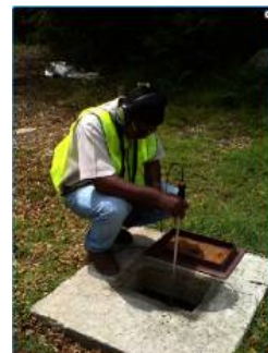
Fig.2 listening directly on a Valve or Hydrant
